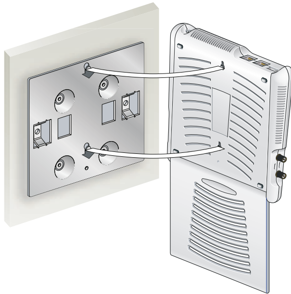
FIGURE 8 Placing the A70 into the Cradle
